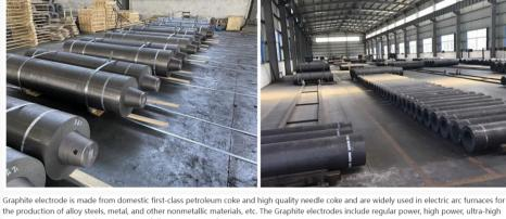
power, and square electrodes. The range of diameters covers from 200mm to 700mm.
